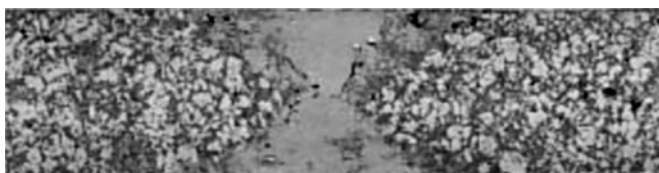
Figure 2. Macroscopic view (filer material: AlMg4.5Zr).
