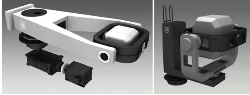
Fig. 1. Centrifuge with 3 degrees of freedom. Fig. 2. SDT with 4 degrees of freedom.
