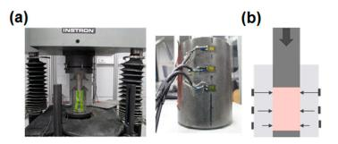
**Figure 2.** (a) Pressing machine used for formation of green bodies, location of radial stress measurements; (b) schematic representation of cylindrical greed body with pressure sensor locations.
