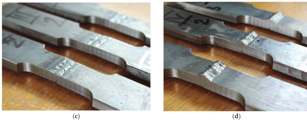
Figure 10. Tensile test specimens with different defect combinations: (a) group I—misalignment, undercut, slight excess root penetration; (b) group II—misalignment, undercut, incomplete root penetration; (c) group III—weld face sagging, incomplete root penetration; (d) group IV—excess weld metal, undercut, incomplete root penetration.
