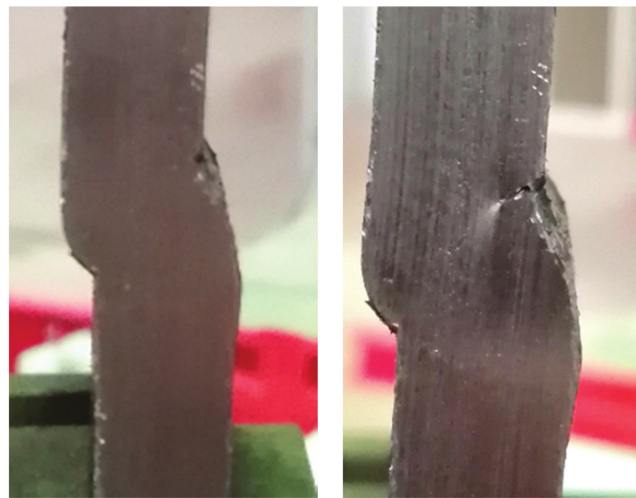
Figure 11. Tensile test specimens during the experiment (misalignment model with slight excess root penetration and undercut) from the initial state to fracture.
