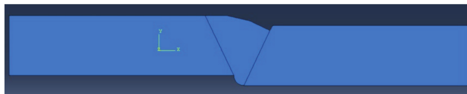
Figure 5. Model with vertical misalignment, undercut, and slight excess root penetration.
