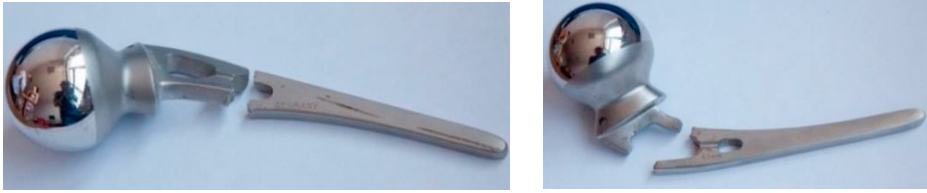
Fig. 5. Typical failures of hip replacement implants
