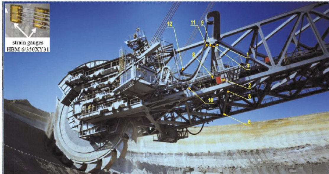
Figure 4. Welded structure of the bucket-wheel boom and spots where strain gauges were located
