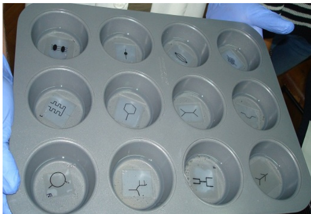
Figure 5. Representative individual microchannel molds in a baking dish, taken from the "Do-it-yourself Microfluidics Workshop", FME UB
