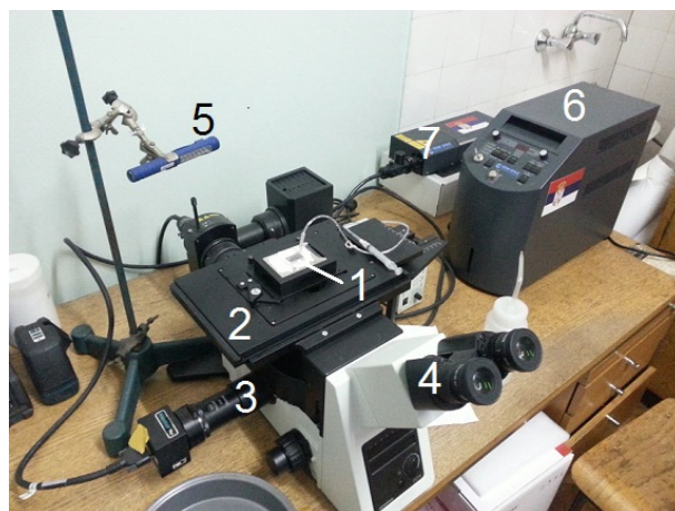
Figure 7. Micro PIV arrangement: 1- microchannel in position for measurements, 2- movable table attached to the microscope, 3- CCD camera, 4- inverted based microscope, 5- LED lamp, 6- laser power supply and 7- dual head Nd:YAG laser
