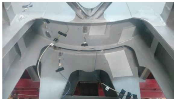
Fig. 3. Parallel measurements using strain gauges and Aramis system
