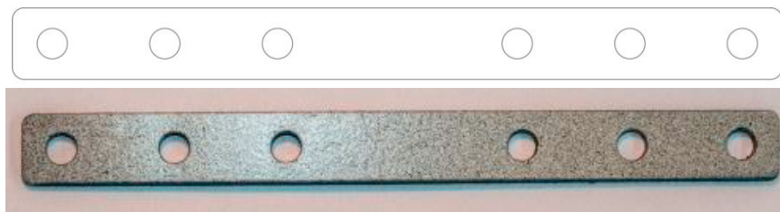
Fig. 1. Schematic of the specimens and prepared Nimonic 263 specimens
