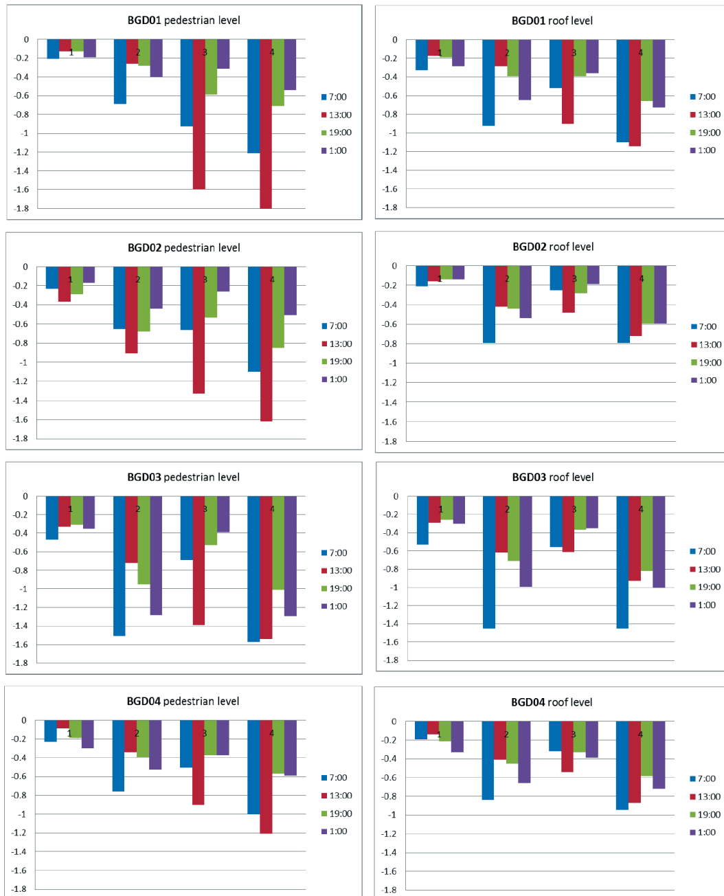
Figure 5. Maximum temperature differences \Delta T [°C] at pedestrian and roof levels predicted by four models in relation to the baseline model at four locations (BGD01, BGD02, BGD03, BGD04) in Belgrade on June 23 at 07:00 h, 13:00 h, and 19:00 h and at 01:00 h on June 24; Legend: y-axis: \Delta T [°C], x-axis: (1) RC+EX green roof comparison with RC, (2) RC+IN green roof comparison with RC, (3) Future comparison with RC, (4) Futureplus comparison with RC
