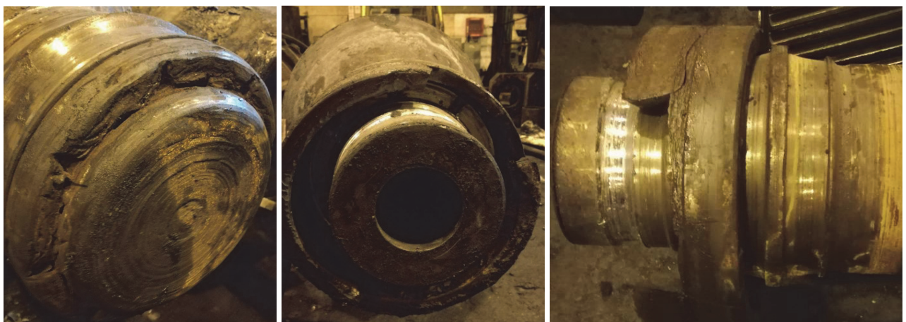
Fig.1. Some of the damages of roller bearings which can (and did) cause the failure of the toothed shaft
