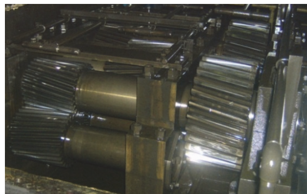
Fig.7. Roller reducers used for flattening of hot-rolled strips during the inspection in 2017
