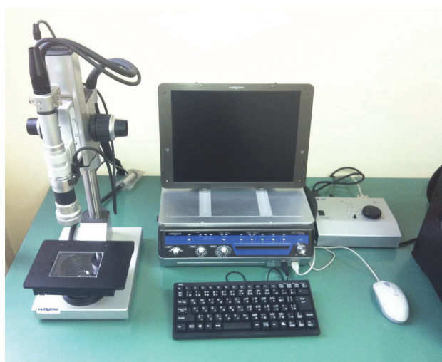
Fig.5. 3D microscope Xirox KH-7700
