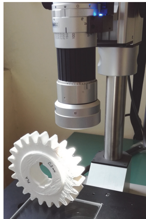
Fig.9. Measuring with 3D microscope
