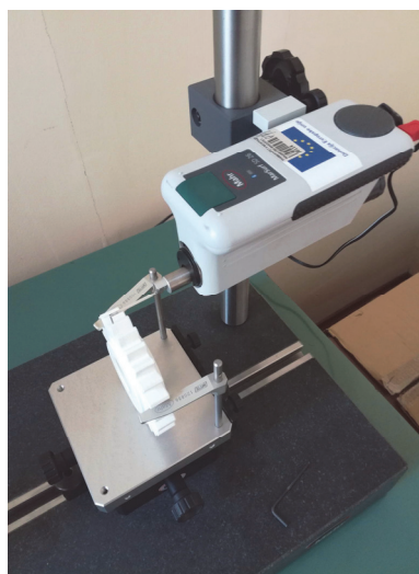
Fig.4. Surface roughness examination Mahr MarSurf SD26
