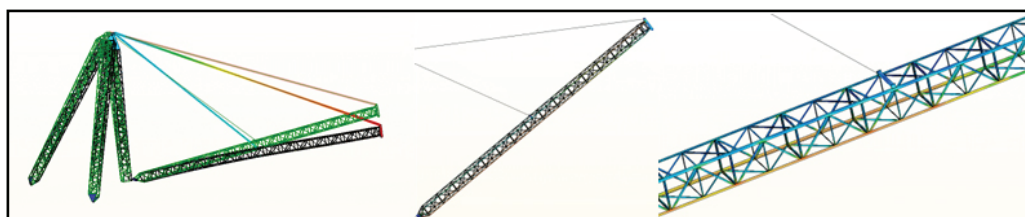
Figure 9: Displacement and Von Mises equivalent stress in the second geometrical configuration (30°)
