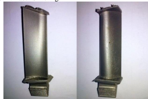
Fig. 5. Photos of considered turbine blade: on the left: pressure side; on the right: suction side
