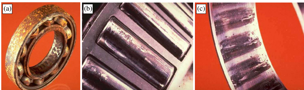
Figure 7. Bearing surfaces damaged by corrosive wear: (a) corrosion pits and rust all over the bearing and (b) and (c) discolouration of contact areas on rollers and outer ring.
