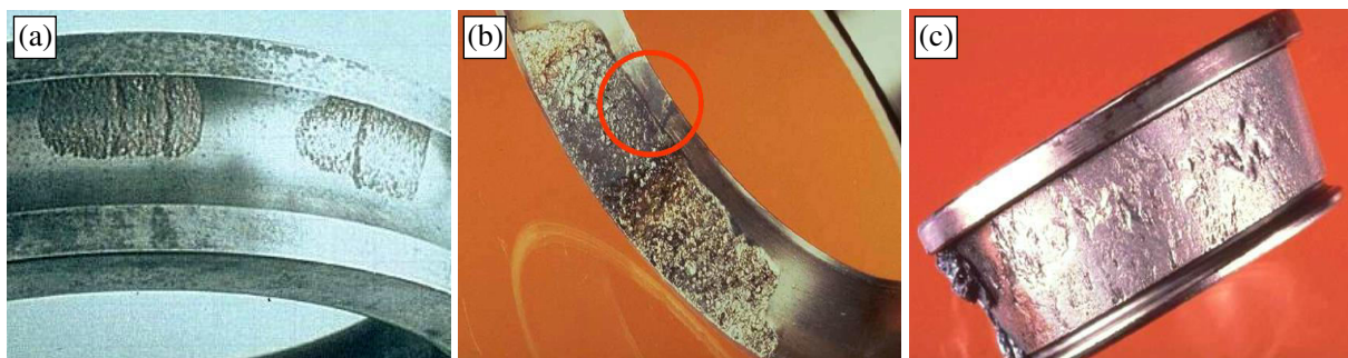
Figure 4. Bearing surfaces damaged by surface fatigue wear: (a) and (b) localised pitting of the inner and outer ring due to overload and (c) progressive pitting of the inner ring due to the inadequate lubrication.
