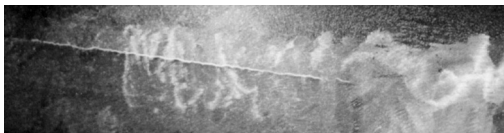
Figure 10. Cracks along fusion line [33].
