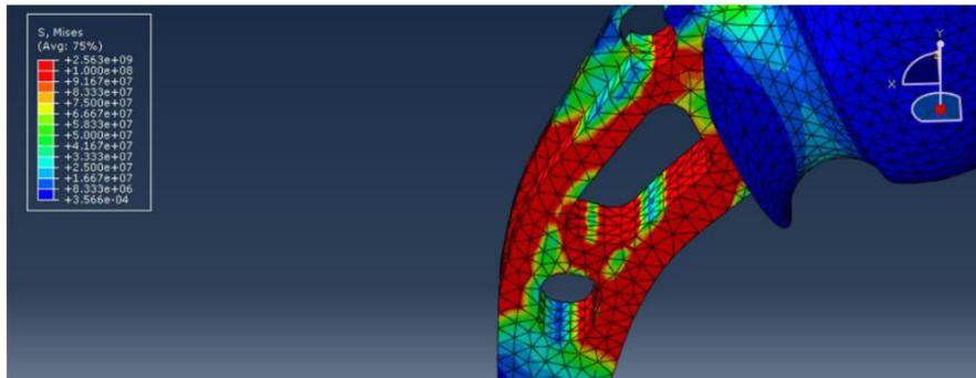
Figure 4. Von Mises stresses in the stem (detailed)
