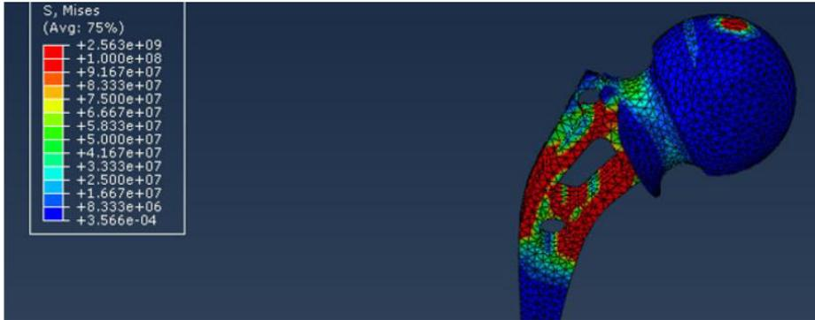
Figure 3. Von Mises stresses in the stem
