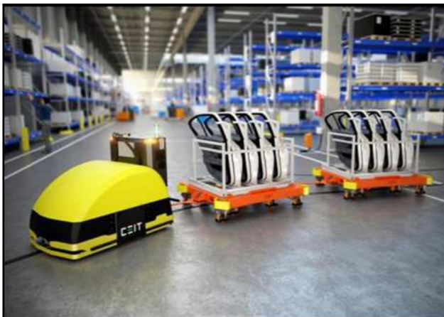
Figure 5: AGV system – towing version
