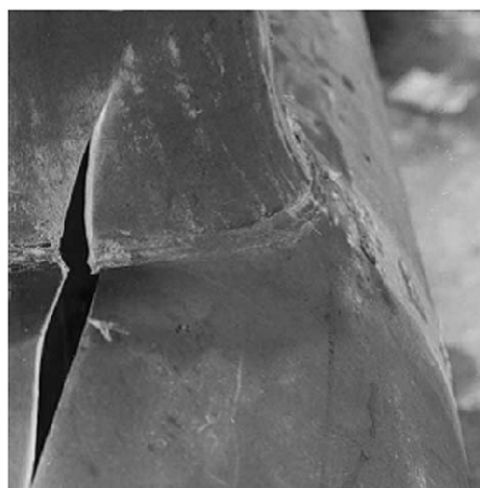
Figure 8. Fractured surface of the test vessel.
