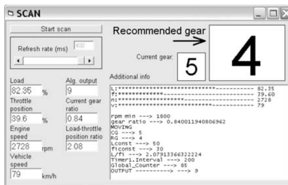
Figure 6. Software output window of the model algorithm with recommended gear
