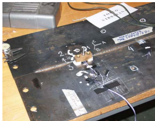
Figure 1. Welded plate, vibrated during welding.
