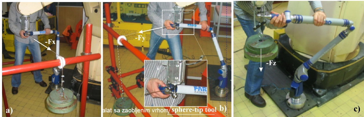
Figure 7. Experimental setup of robot loading and displacements measurement
