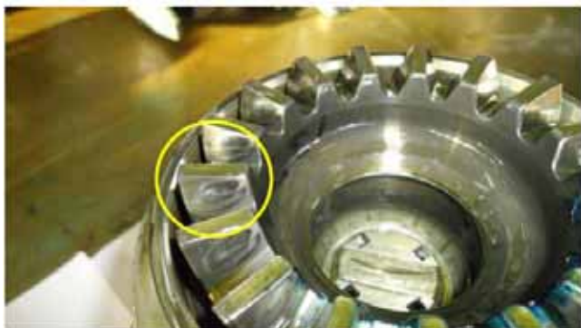
Figure 9. The surface damage on the gear wheel of the inter gear box of the Gazelle helicopter
