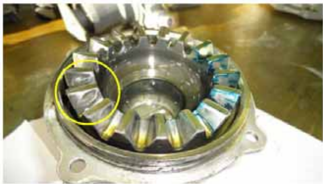
Figure 8. The surface damage on the gear wheel of the inter gear box of the Gazelle helicopter
