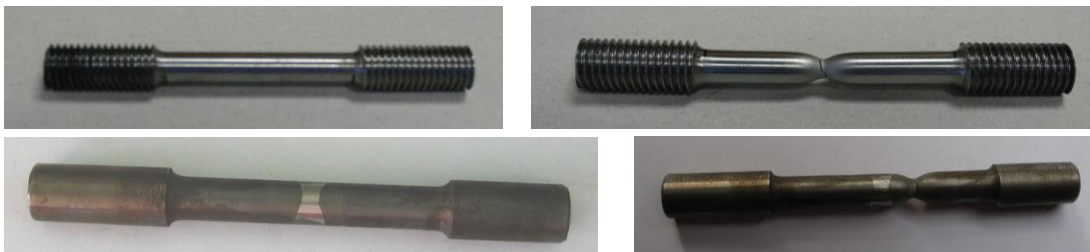
Fig. 2. Test samples appearance: upper figures BM sample before (left) and after (right) the test; lower figures: weld metal sample before (left) and after (right) the test.
