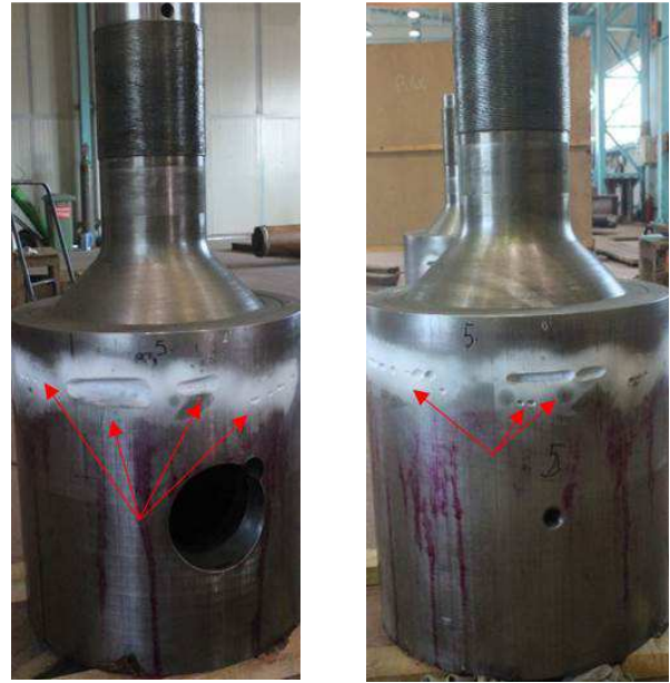
Figure 4. Preparation of surfaces for the repair (body of the glass nr. 5)
