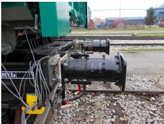
Fig.7. Buffing impact test – wagon end with installed force and displacement transducers [8]
