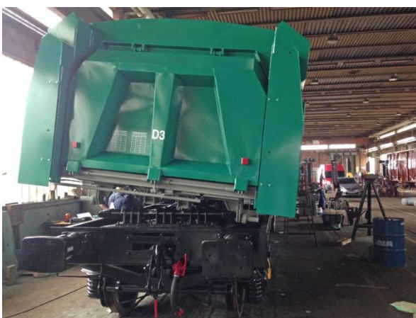
Fig.3. Lateral tilting of the cargo crate for side discharging
