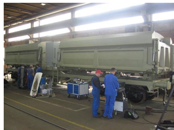
Fig.4. Stationary brake test [4]
