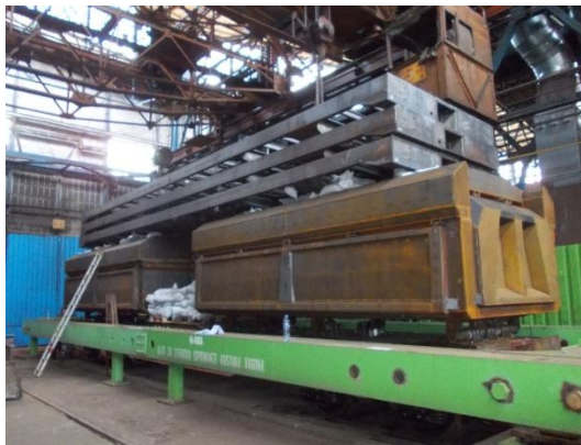
Fig.6. Carbody static strength test [6]
