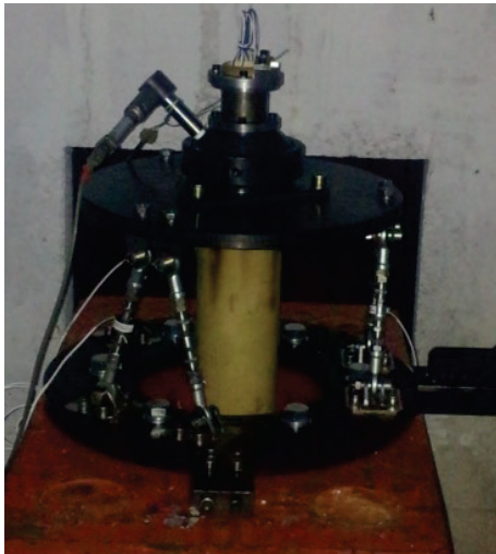
Figure 24 Motor at six-component test stand at EDePro company site
