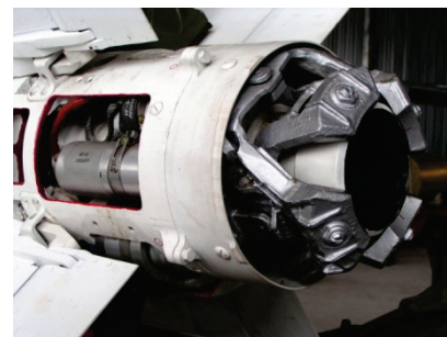
Figure 3 Segmented dome deflector at solid rocket motor nozzle (R73 air to air rocket)
