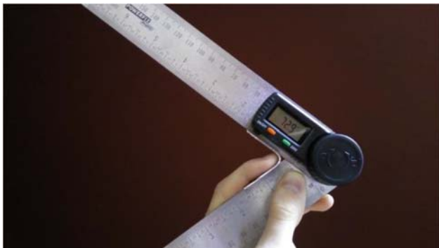
Fig. 5 Measurement of achieved bending angle.
